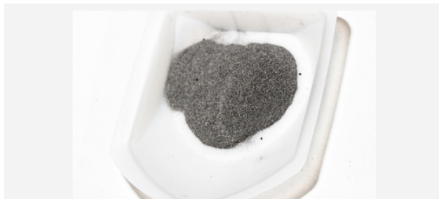
Researchers have created molten air batteries using iron, carbon and vanadium boride because of their ability to transfer multiple electrons. These batteries can store three, four and 11 electrons per molecule respectively, giving them 20 to 50 times the storage capacity of a lithium battery, which can only store one electron per molecule of lithium.
