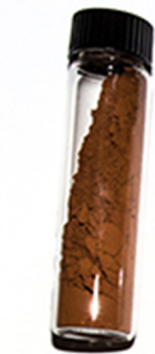
Electrolyte \text{Fe}_2\text{O}_3 in eutectic carbonate
